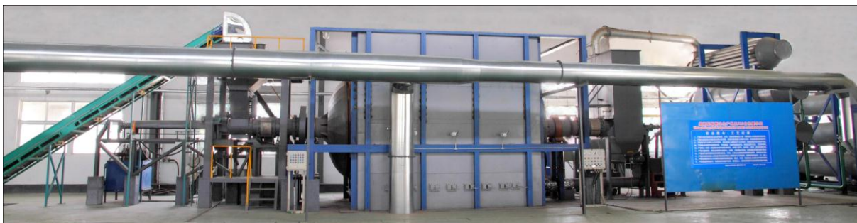
Automated continuous plastic to liquid fuel process (Source: PARC )
