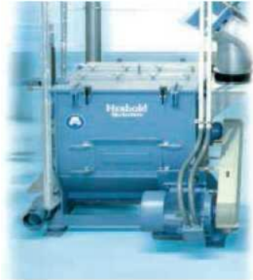
Figure 3: Intensive wet washing and hydrocyclone technology (Source: Herbold Meckesheim GmbH)
